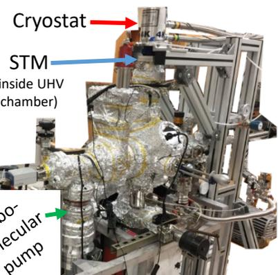
1. The cryostat brings the working environment to 10K.
