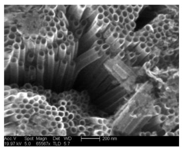
Nano-particles formed in the shape of tubes and made of anatase are used in solar-panel research.
